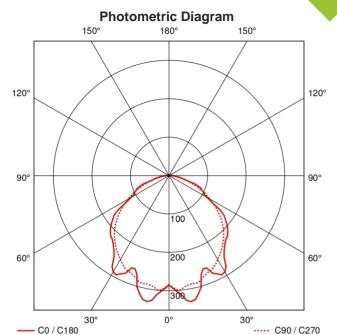
cd / 1000 lm Luminaire Efficiency: 89.2%
