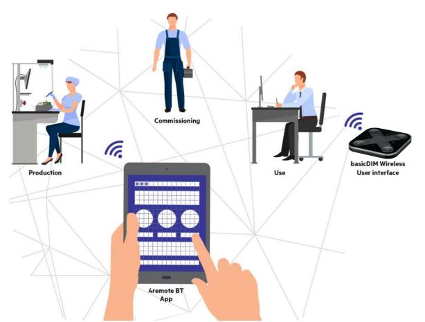
Bluetooth Wireless control technology allows versatile and processional interaction with all luminaires within an area - fully intuitive and with no additional wiring required.
